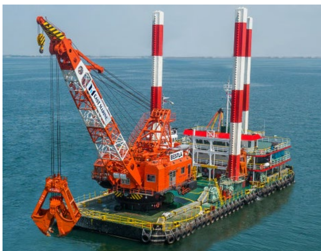
10m 3 Grab Dredger "Bestla" (East Marine, 2014).
